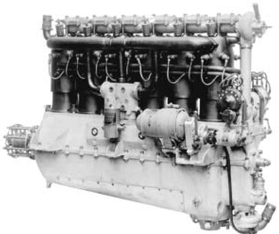
In Friz's design the cylinder head and cylinders formed one inseparable unit, with the steel cylinder liners simply being bolted into the cylinder head extending far down into the engine block itself. In this way Friz was able to do without a cylinder head gasket. Dry sump lubrication and dual ignition gave a reliable and consistent supply of oil and kept the engine running reliably at all times.
